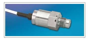
the sensor. For applications where a true flush diaphragm is needed, Kulite will supply these transducers without the screen. Incorporation of a Kulite proprietary electronics module within the main body of this product allows for operation from an unregulated power supply of 12  $\pm$  4 VDC or 28  $\pm$  4 VDC. Standard output is a stable, low noise 0 to 5 VDC signal.
